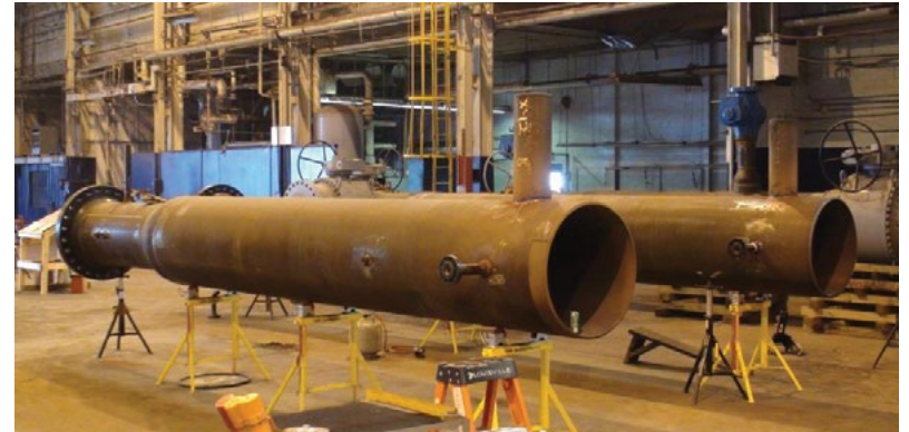
Pipeline Inspection Gauge Launcher/Receiver Barrels
