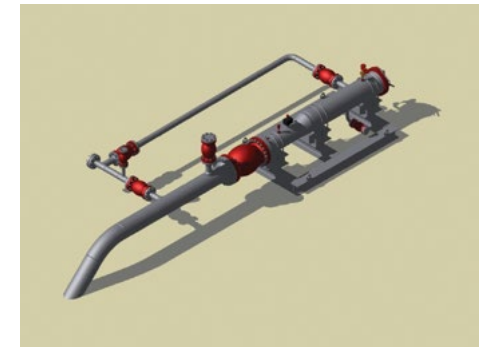
Pipeline Inspection Gauge Launcher
